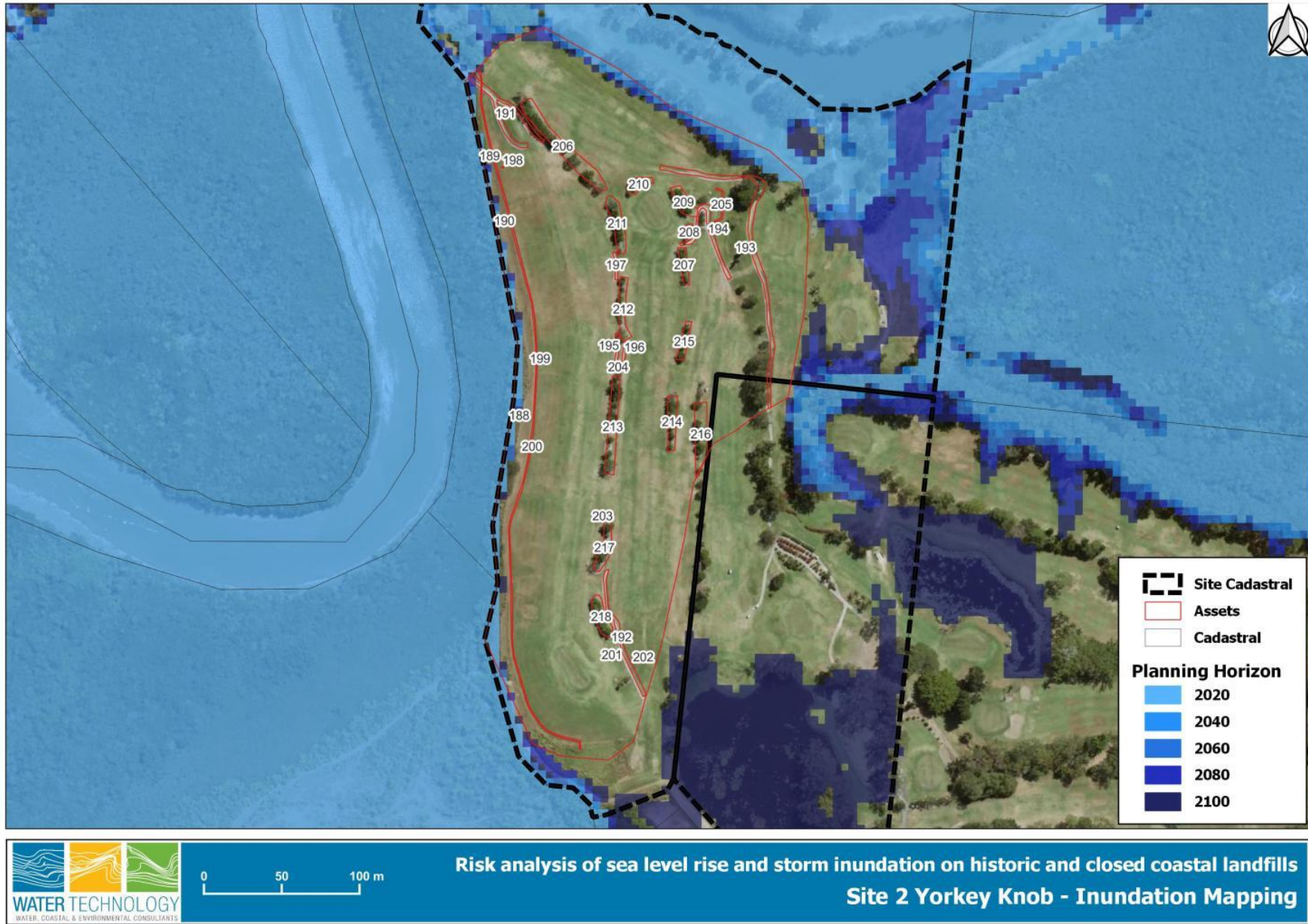
Figure C-3 Yorkeys Knob Site – Coastal Inundation
